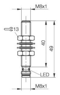
**Inductive Sensors** BES M08EG-PSC15A-S49G-W M8 x 49 normally-open Sn=1,5mm shielded Factor 1
